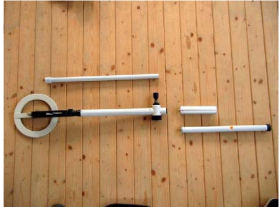
The detector with the modular extension (above) and the two possible power attachments (right). The armrest and handle are not displayed
