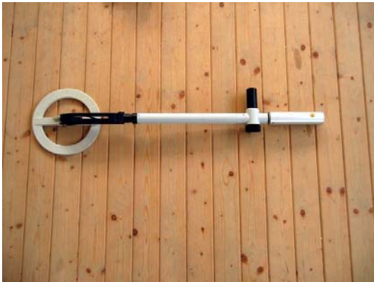
The detector in short configuration with the rechargeable battery pack. The armrest and handle are not displayed
