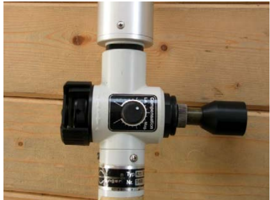
Sensitivity knob (left), soil compensation adjustment knob (middle), and loudspeaker (right) which can be covered by a protective cylinder.
