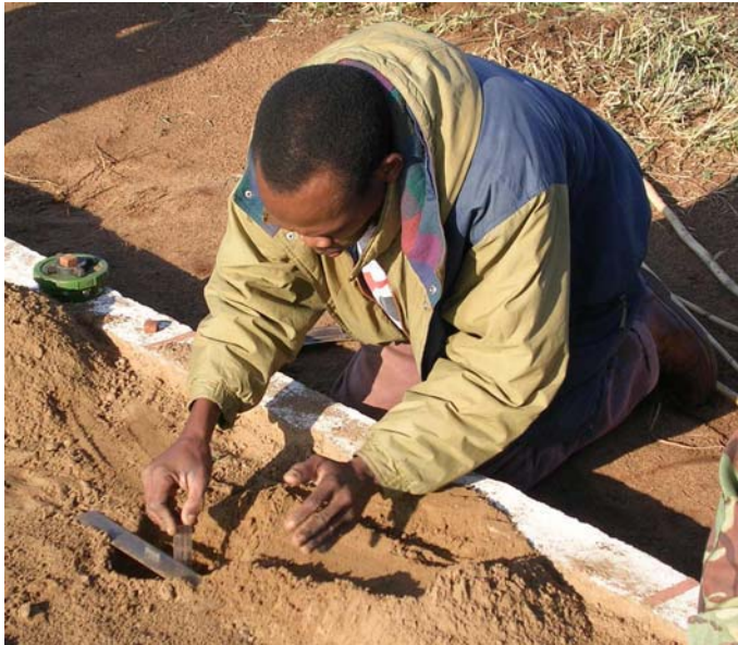
Plate 5-7 Filling of the hole and depth measurement of the target
